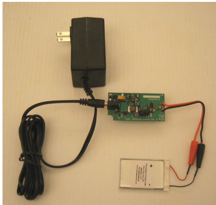
Figure 2. AC12050615A-01 shown with no enclosure and a 5VDC, 1.0A voltage supply charging a 1000mAh Advantage Circuits polymer-lithium-ion battery.
